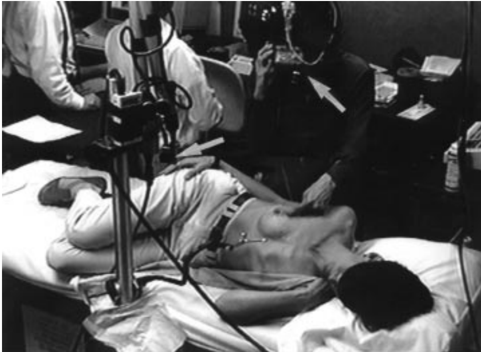
Fig. 3. Preliminary human subject experiment. The physician (EDP), wearing an HMD (marked by top-right arrow) is examining the subject's right breast. The left arrow points to PIE Medical 7.5 MHz ultrasound transducer, attached to FARO Technologies mechanical arm for precise 6 degree-of-freedom tracking. This has been replaced by a less cumbersome system using a Flashpoint 5000 3D localizer to track the transducer without encumbering the physician.
