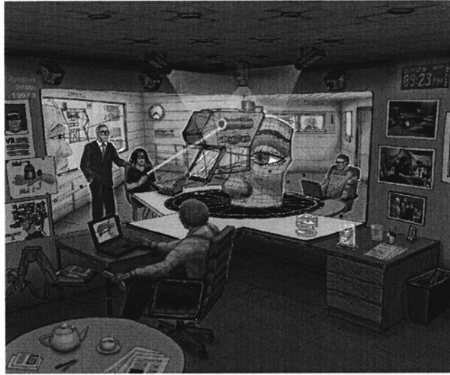
Figure 1.5: This drawing, by Andrei State of UNC-Chapel Hill, shows a view of the Office of the Future. Large displays (provided by the projectors mounted in the ceiling), cover the walls and desk. The user is able to participate in a discussion with his colleagues who appear to him as sitting on the other side his desk. He is able to use his personal computer to make notes while working collaboratively on a design for a new head mounted display, which appears to be hovering over his desk. ( c)1998, Dept. of Computer Science, UNC-Chapel Hill )
