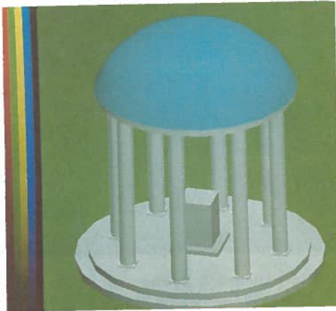
Fig. 5: The Chapel Hill "Old Well" rendered by a Pixel-Planes functional simulator with input of 357 polygons. Estimated image generation time (assuming a 10Mhz clock) is 9 msec.
