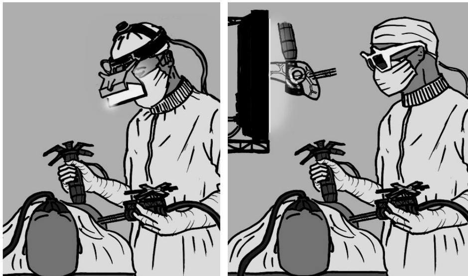
**Figure 3.** Display modalities under consideration for the RFA 3D guidance system, both using optoelectronic tracking (overhead). Left: ST-HMD provides virtual image inside of and registered with the patient (cf. Fig. 1, right). Right: fish tank VR system shows 3D virtual image above patient (cf. Figure 4).
