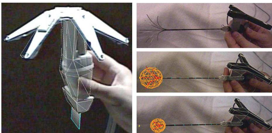
**Figure 2.** Left: ST-HMD view of ultrasound transducer with infrared LEDs for motion tracking. Note ultrasound image below transducer. Right, top to bottom: motion-tracked RFA probe with deployable tines and real-time registered guidance graphics. The ablation region (sphere) is scaled based on current tine length.
