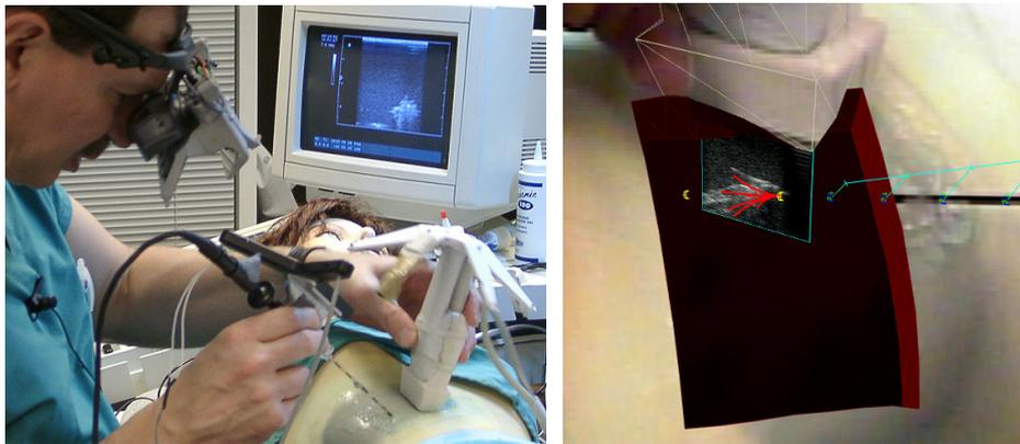
**Figure 1.** Left: RFA guidance system with see-through head-mounted display. Right: view inside HMD with 3D guidance graphics indicating relationship between needle-like RFA probe and ultrasound image plane.
