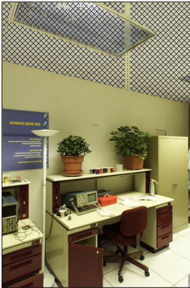
Figure 4. The ceiling over the workbench is highlighted with a pattern, indicating that the ceiling was the “strongest” planar area in a 3D-Hough transform of the range data. Finding and matching planar areas in different scans is one way of determining the rigid-body transformation between two scans.
