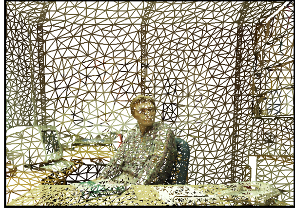
Figure 6. On the left is a view of the immersive telecollaboration setup. The person in the office is viewing a stereo image of one of our 3D models of an office in our department. The person is tracked (device on head) to accurately update the display as he moves. The scene "through the window" is static in this image, but there are results with real-time reconstruction of participants over the network.
