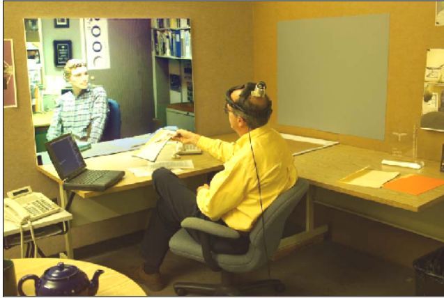
Figure 6. On the left is a view of the immersive telecollaboration setup. The person in the office is viewing a stereo image of one of our 3D models of an office in our department. The person is tracked (device on head) to accurately update the display as he moves. The scene "through the window" is static in this image, but there are results with real-time reconstruction of participants over the network.
