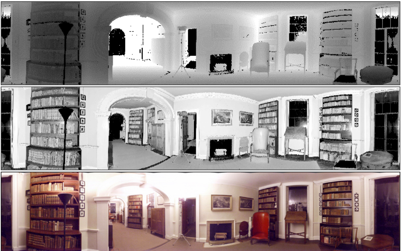
Figure 1. Examples of our data. The scene is Thomas Jefferson's library at Monticello, VA. The top image is a range map, where lighter is further (black is no data), the center image is the reflected laser light image, and the bottom image is the color panorama taken from the same point.
