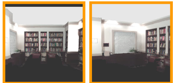
Figure 10. Two views of a library represented by 10 triangles with relief texture maps. The per-pixel relief allows proper motion and occlusion of the scene.
