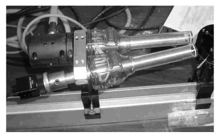
Figure 1: our structured light depth extracting laparoscope prototype shown with surgical trocars (laparoscopic access ports, Ethicon Endopath® 18mm) over the laparoscope tubes. The miniature projector is attached to the upper laparoscope, and a camera is attached to the lower laparoscope
