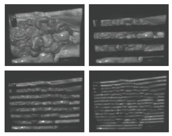
Figure 3: Sample images acquired from the abdomen of a porcine cadaver using a large projector to project stripe patterns onto the organs. The image in the upper left shows the abdomen fully illuminated. High intensity spots on the surface are the result of specular highlights.
