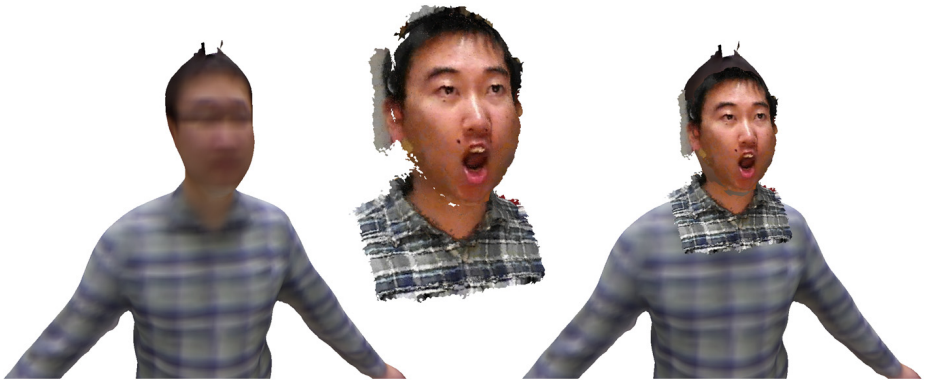
Fig. 4. The base surface from the RGB-D frames from multiple static Kinect cameras (left), the stereo reconstruction from the high resolution PTZ cameras (center) and the final fused surface (right)
