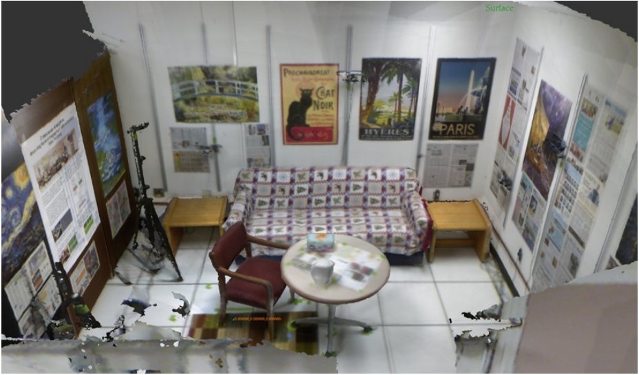
Fig. 1. The 3D surface of the static background using only RGB-D frames from a single moving Kinect. The surface is a color-by-vertex model and lacks detail.
