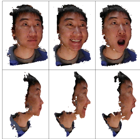
Fig. 3. The 3D point clouds obtained using only images from the PTZ cameras. These point clouds represent the union of three distinct point clouds, and then fused using known camera parameters of the PTZ cameras.
