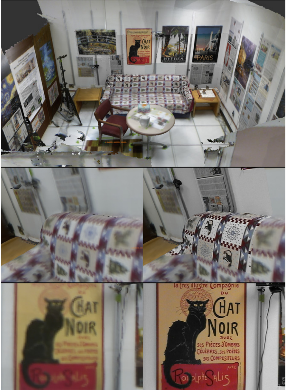
Fig. 2. The final output of texture transfer from PTZ images. We show regions of high-resolution texture against the low-resolution surface generated from images from a single moving Kinect. We report an approximately 6x improvement in texture quality, measured as color sample per unit area, in areas where the texture was transferred as compared to where it was not.
