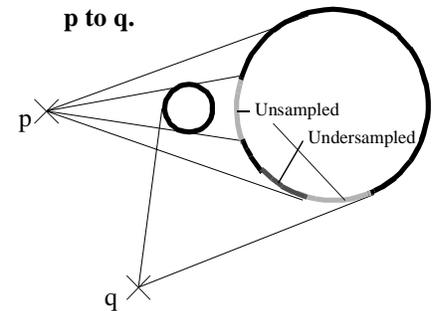
Figure 2: A sufficient set of views is found by intersecting the viewing rays with the sampling sphere.
