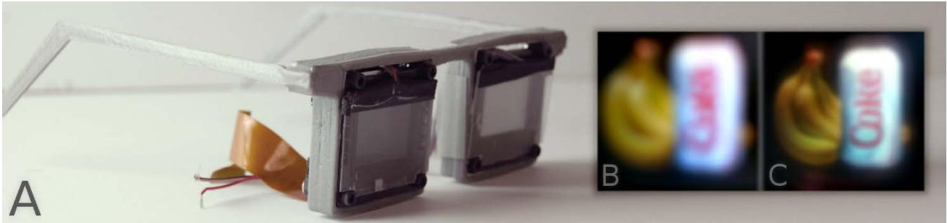
Figure 1: A) Prototype optical-see through glasses with a wide field of view and occlusion support. (Driving electronics are external.) The device is capable of providing in-focus augmented images at multiple simultaneous focal depths using only a set of backlit stacked LCD panels placed closer than the eyes can accommodate: the distance of normal eyeglasses. B,C) Photos taken of a prototype display with a 3.7 mm lens aperture and a distance of 18 mm between the display and the camera's center of projection, approximating a human viewer wearing eyeglasses. The camera focus distance was set to 10 cm. Photo B) was taken with an image naively displayed on one of the layers, while photo C) was taken using the multilayer optimization technique described in this paper.
