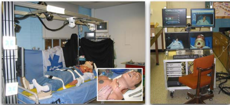
Figure 14: Left: modified Portable Camera Unit (c.f. Figure 11) positioned over the Human Patient Simulator; inset shows a close-up of the access for difficult airway management. Right: 2D videoconference station for the remote physician.
