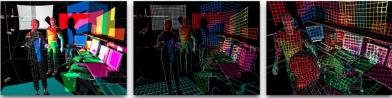
Figure 15: Multi-camera visibility simulator. Left: the cameras (floating cylinders at the left) are treated as flat-field colored lights. Center: the same view with projected grids to show each camera’s imaging resolution. Right: a close-up showing camera visibility overlap areas.
