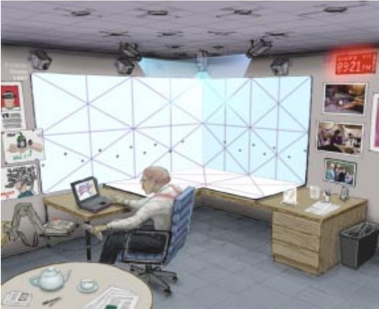
**Fig. 2.** The Office scene during projector calibration procedure, showing the results of automatic blending of overlapped projected image regions.
