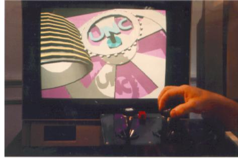
Images from Pixel-Planes 4 illustrating direct rendering of spheres and shadows.
