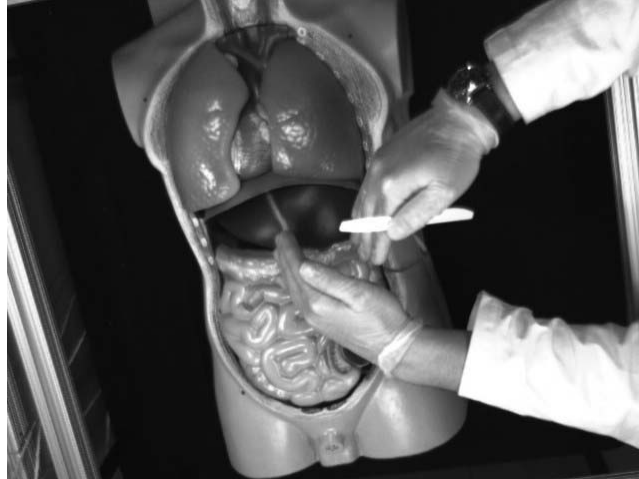
Figure 5: Specular highlights are visible in this image from a surgical training mockup and would be even worse in a real surgical situation.
