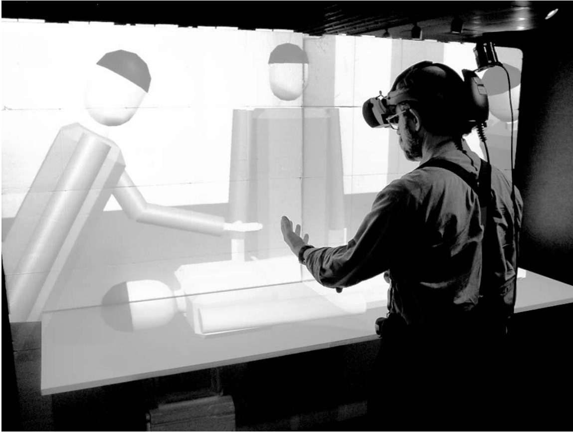
Figure 6: The hybrid display consists of a head-mounted display and several wall-based projectors.
