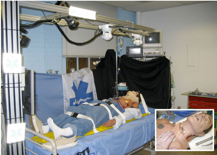
Fig. 8.7 Human patient simulator (HPS) staged as an accident victim for the experimental evaluation. Note the 2D video cameras and display mounted on the overhanging structure. Inset shows the HPS airway details
