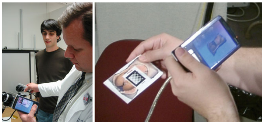
Fig. 8.5 Left: Our first tracked PDA prototype used a HiBall-3000™ tracking system [1], with sensors mounted on the PDA (Toshiba e800, left hand ) and the surrogate ( right hand ). Right: Our current prototype uses a PointGrey DragonFly camera [3] mounted on the PDA ( left hand ). The prop ( right hand ) has a printed image of our training torso on it, along with a grayscale pattern. We use the ARToolkit [2] to track the surrogate with respect to the PDA (camera)
