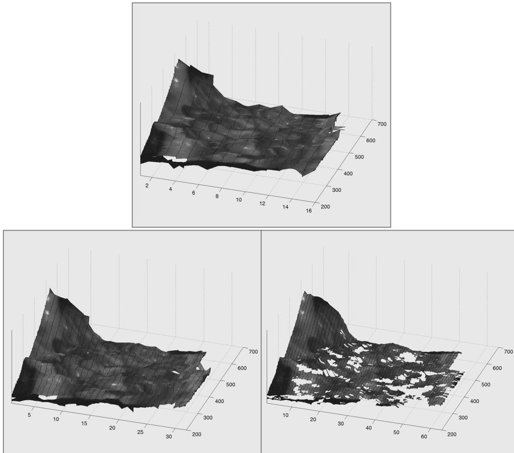
Figure 4: These three images show range images calculated from images with stripes projected onto the abdomen of a porcine cadaver. The stripes were identified using our method. These images show a progressively increasing number of stripes (top to bottom, left to right). In the image calculated with the largest number of stripes, large holes appear because aliasing of the stripes prevented their identification.
