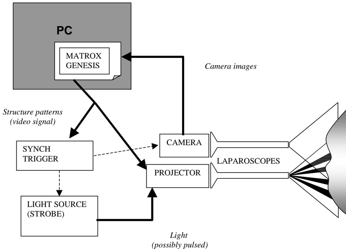
Figure 2: A schematic overview of our system for laparoscopic depth extraction. The Matrox Genesis board in the PC outputs the structured light patterns as a video signal to the miniature projector. This video signal can also be used to trigger synchronization signals for the projector's light source and/or the camera. The images acquired by the camera are captured and processed by the Matrox Genesis board.
