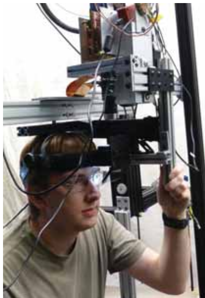
Fig. 2: A user “wearing” our AR Display. The monocular virtual imagery is presented to the user’s left eye.
